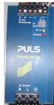
Puls Dimension QS10.DNET Power Supply
